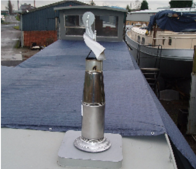
FIG 7 MK3 FLUE FITTED TO A LUXE MOTOR WITH DYNAMIC TYPE SWEEP VENTURI COWL.
